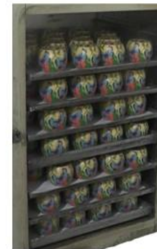
9. The finished product is baked in an oven to harden the clay and complete the production process
